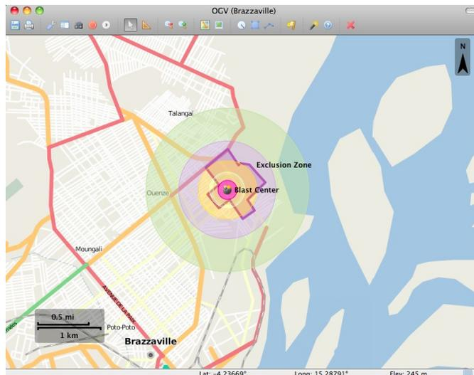
Figure 5. Brazzaville, Congo munitions depot explosion of March 4, 2012 showing damage rings based on reports and blast calculator tool.
